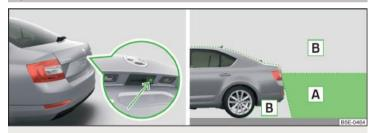
Fig. 162 Position of the camera / Monitored area
