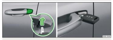
Fig. 232 Handle on the driver's door: covered locking cylinder/locking cylinder with key
