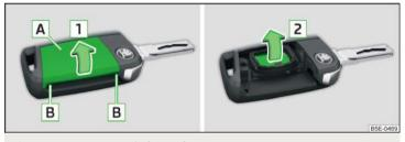
Fig. 230 Remove cover/take out battery
