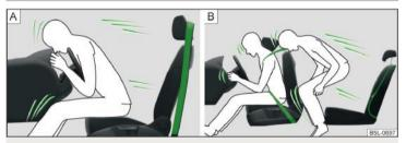
Fig. 4 Driver without a fastened seat belt/rear seat passenger without a fastened seat belt
