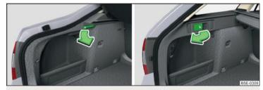
Fig. 82 Fold the backrest forward from the luggage compartment: Variant 1/variant 2
