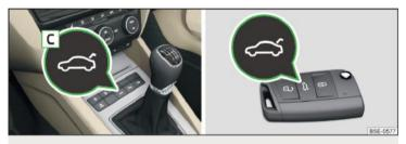
Fig. 46 Button for the lid operation / button on the key
