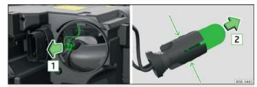
Fig. 246 Headlights with Xenon light: Bulb for additional parking light
