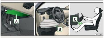
Fig. 10 Installation of the airbag / Gas-filled Airbag / Safe distance between the legs and the instrument panel
