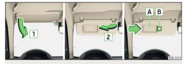
Fig. 66 Fold down visor / flip up visor / make-up mirror and Park Memo Holder
