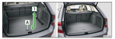
Fig. 126  $\,$  Set variable loading floor to the upper position / variable loading floor in the upper position
