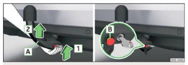
Fig. 189 Insert ball rod / trigger bolt in the extended state
