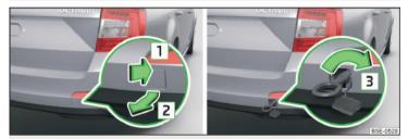
Fig. 228 Expansion of the cap / installation of towing eye - Version 1
