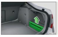
Fig. 122 Remove storage compartment
