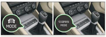
Fig. 176 Button for selecting the driving mode: Version 1 / version 2
