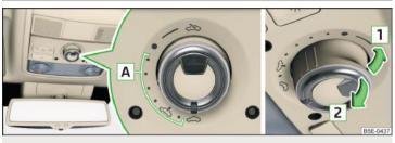
Fig. 50 Operation of the sliding/tilting roof - Version 1
