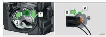
Fig. 244 Headlight with halogen bulb: Bulb for low beam
