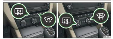
Fig. 65  $\,$  Buttons for the front and rear window heater: manual air conditioning, heating / Climatronic
