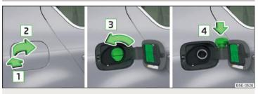
Fig. 199 Open fuel filler flap/unscrew tank cap/place the tank cap on the fuel filler flap
