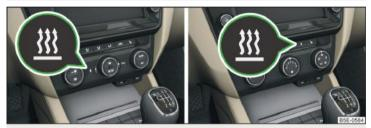
Fig. 140 Button for direct power on / off of the auxiliary heating (heating and ventilation) on the front panel of the Climatronic / manual air conditioning
