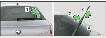
Fig. 237 Rear window wiper blade
