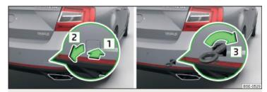
Fig. 229 Expansion of the cap / installation of towing eye - Version 2
