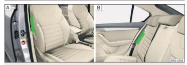
Fig. 11 Installation locations of airbags: in the front seat/the rear
