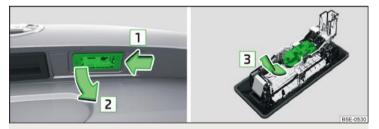
Fig. 249 Remove the number plate light/replace the bulb
