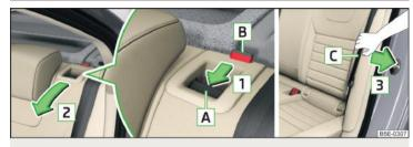
Fig. 81 Fold the seat backrest forwards from the interior/pull the belt for the side trim
