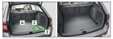
Fig. 127 Set variable loading floor to the lower position / variable loading floor in the lower position
