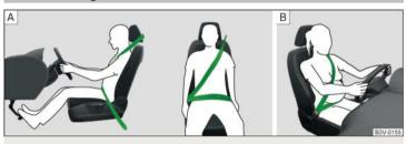
Fig. 5 Routing of belt webbing over the shoulders and the lap belt/Routing of belt webbing for an expectant mother
