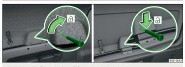
Fig. 234 Unlocking the boot lid: Version 1 / version 2
