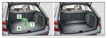
Fig. 128  $\,$  Fold up variable loading floor / folded variable cargo floor in the upper position
