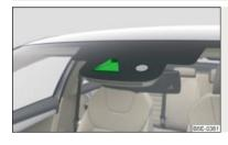
Fig. 181 Camera viewing range for traffic sign recognition
