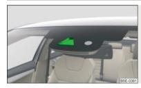
Fig. 57 Camera view window for the main beam assistant
