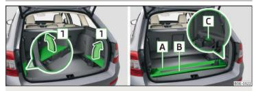
Fig. 134  $\,$  Remove the side panels of the luggage compartment/stow the roof rack
