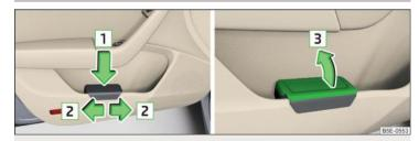
Fig. 93 Waste container: inserting and moving/opening
