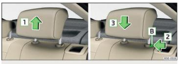
Fig. 74 Rear headrest: moving up/down
