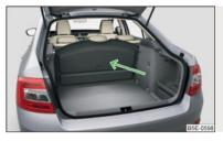
Fig. 119 Luggage compartment cover stowed behind the rear seats
