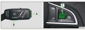
Fig. 30 Buttons/dial: on the control lever/multifunction steering wheel
