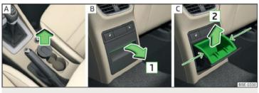
Fig. 91 Remove front ashtray / open rear ashtray / remove rear ashtray insert
