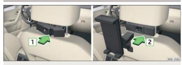
Fig. 105 Position adapter/install holder
