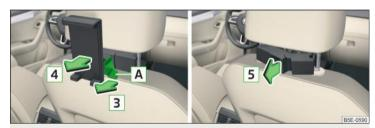
Fig. 106 Remove holder/remove adapter
