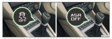
Fig. 155 System button: Vehicle with ESC / vehicle without ESC
