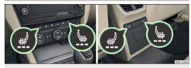
Fig. 77 Buttons for heating the front seats/rear seats
