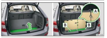
Fig. 124 Lift floor covering/storage compartments under the floor covering
