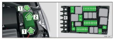
Fig. 241 Removing the fuse box cover/fuses
