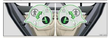
Fig. 42 Rear door: Child safety system switch on / off
