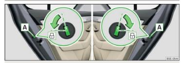
Fig. 233 Emergency locking: Left/right rear door
