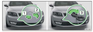
Fig. 227 Removing the cap / installing the towing eye
