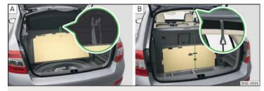
Fig. 116 Fixing the floor covering: Version 1 / version 2
