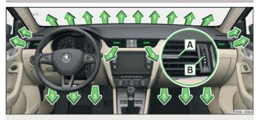
Fig. 138 Air vents at the front
